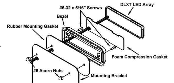
3. Mount the DLXT light(s) on the bracket as shown above. Use the two #6-32 x 5/16" screws through the back of the mounting bracket as shown. Secure the screws using the two #6 acorn nuts. Repeat for additional lights, if applicable.
